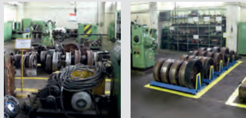
Heavy Section Mill workplace before and after 5S implementation
